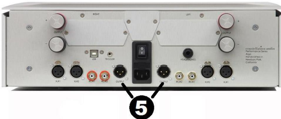
The two inner XLR connections on the rear of the Argo are outputs. These can be connected to a larger, more power amplifier such as the Constellation Audio Hercules or Centaur. They can also be connected to a system in a second room, or to a powered subwoofer.
