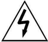
The lightning flash with arrowhead, within an equilateral triangle, is intended to alert the user to the presence of uninsulated "dangerous voltage" within the product's enclosure that may be of sufficient magnitude to constitute a risk of electrical shock to persons.
