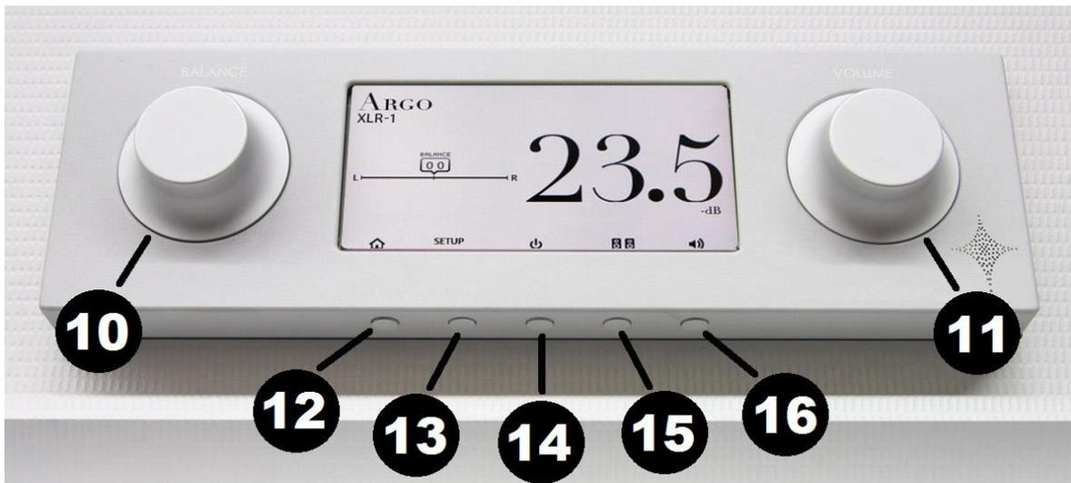
The front panel includes an LCD touchscreen and two knobs plus five buttons positioned underneath the display. These buttons allow you to control the Argo without its remote. The functions of the buttons are shown using icons on the touchscreen. Here are the functions of the buttons and knobs:
