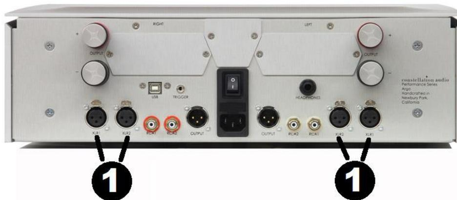
On the rear of the Argo integrated amp are four XLR inputs, two on each side. As you are looking at the rear panel, the left two XLR inputs are for the right channel, the right two inputs are for the left channel. Underneath each jack is the corresponding input number. Use of XLR connections is recommended for the best possible audio quality. To remove an XLR plug, push on the tab above the jack and pull the plug out.
