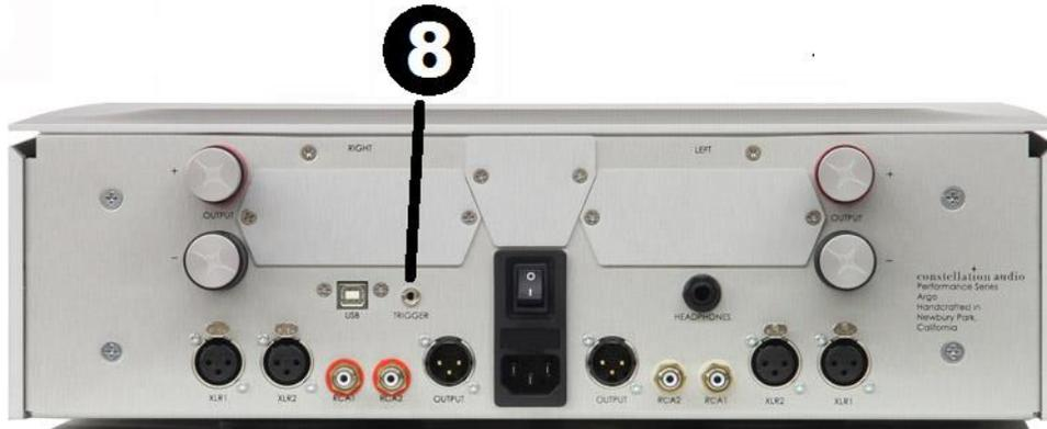
This 1/8-inch/3.5mm jack outputs a 12-volt DC trigger signal when the Argo is powered on. This signal can be used to automatically turn on a connected amplifier (if the amp has a DC trigger input), or to trigger home automation systems.
