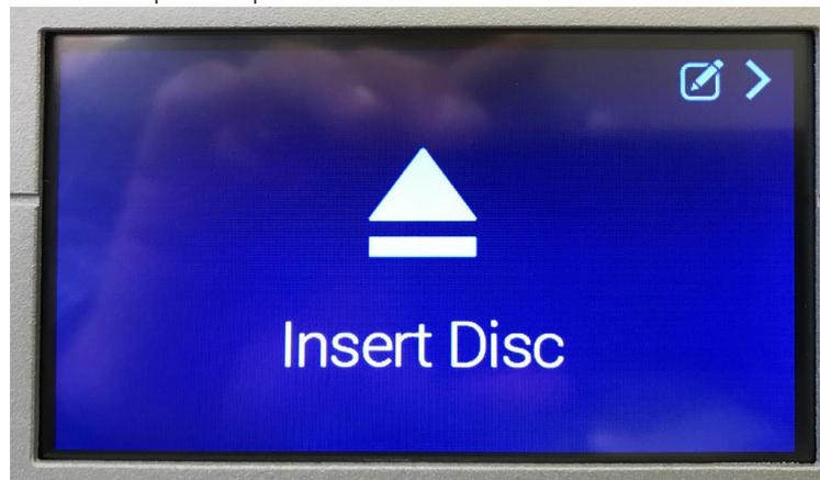
The drawer opens. Insert a disc, label side up and facing you. A slight nudge to the drawer will close it, or repeat the touch to the drawer icon or remote control to close the drawer.
