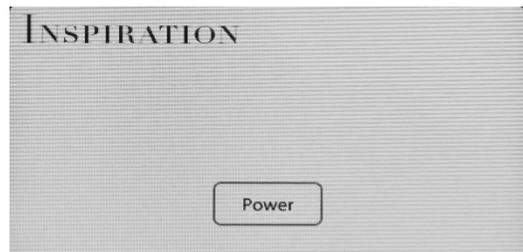
When you turn on the power, you will hear the PREAMP 1.0's internal relays click as the unit goes into warm-up mode. In a few seconds, the front touchscreen will illuminate. The most recently used input will be selected. If you wish to let the unit warm up for a while before listening, hit the Standby button (on the front panel or remote) again to enter Standby mode. The Standby screen will appear on the LCD and the audio will be silenced until you push the Standby button again.
