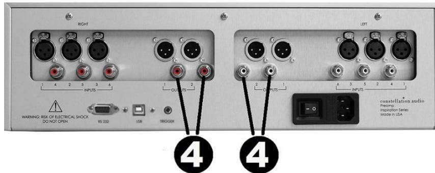
RCA unbalanced outputs are supplied for amps and recording devices not equipped with XLR inputs. The signal at these outputs is the same—it does not matter if you use output 1 or output 2. From left to right, looking at the back of the PREAMP 1.0, the outputs are: 1<sub>right</sub>, 2<sub>right</sub>—2<sub>left</sub>, 1<sub>left</sub>.
