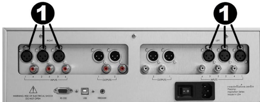
On the rear of the PREAMP 1.0 there are six XLR inputs, three on each side. As you are looking at the rear panel, the left three XLR inputs are for the right channel, the right three inputs are for the left channel. Underneath each jack is the corresponding input number. Use of XLR connections is recommended for the best possible audio quality. To remove an XLR plug, push on the tab above the jack and pull the plug out.
