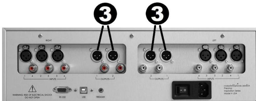
The inner four XLR connections on the rear of the PREAMP 1.0 are outputs. The signal at these outputs is the same—it does not matter if you use output 1 or output 2. To remove an XLR plug, push on the tab on the connector body and pull the plug out.
