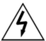
The lightning flash with arrowhead, within an equilateral triangle, is intended to alert the user to the presence of uninsulated dangerous voltage within the product enclosure that may be of sufficient magnitude to constitute a risk of electrical shock to persons.
