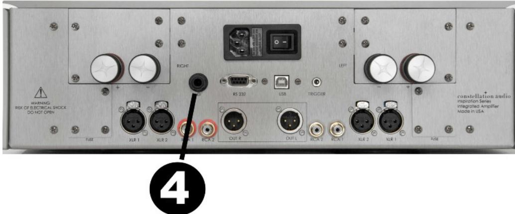
The Inspiration Integrated offers a single headphone output on a 1/4-inch (6.3mm) jack. To activate this output (and mute the speaker outputs), you must use the front-panel controls. The Inspiration Integrated's headphone amplifier has enough power to drive any dynamic or planar magnetic headphones. If your headphones have a 1/8-inch (3.5mm) plug, use a 1/8-inch to 1/4-inch adapter. Many headphones come with the adapter.
