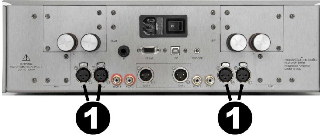
On the rear of the Inspiration Integrated are four XLR inputs, two on each side. As you are looking at the rear panel, the left two XLR inputs are for the right channel, the right two inputs are for the left channel. Underneath each jack is the corresponding input number. Use of XLR connections is recommended for the best possible audio quality. To remove an XLR plug, push on the tab above the jack and pull the plug out.
