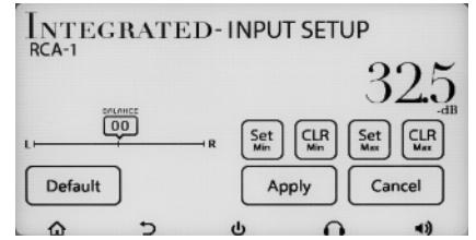
To set up a home theater bypass input: First select the input you want to use for this function, then adjust the volume on the Inspiration Integrated to the desired level. Push the Set Min button, then the Set Max button, then the Apply button. To clear these settings, press CLR Min then CLR Max, or press Default.
