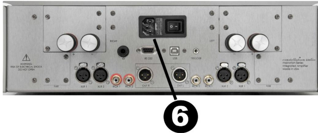
This jack accepts a standard 15-amp IEC AC connector. You can use the AC cord supplied with the Inspiration Integrated, or substitute your own cord. Before making this connection, turn the power switch above the AC input off. Connect the AC cord to the Inspiration Integrated, then plug the AC cord into the wall or your power conditioner, then turn the amplifier's power switch on.
